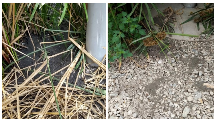
Figure 4: sludge deposition during 3 rd phase on the line with layer (left) and on the line without layer (right)
