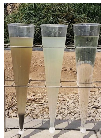
Figure 3: Samples of Raw Wastewater and Effluent of the 1 st stage and 2 nd stage
